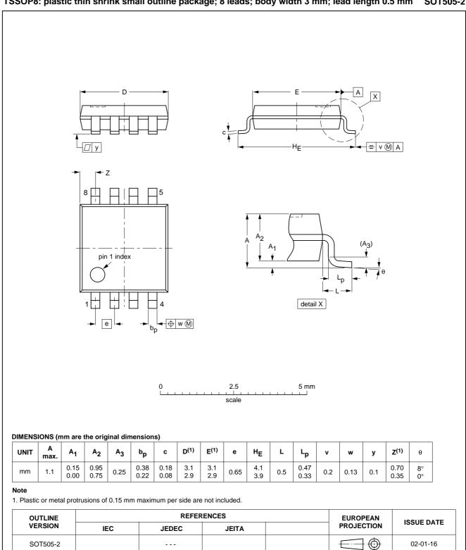
TSSOP8: plastic thin shrink small outline package; 8 leads; body width 3 mm; lead length 0.5 mm SOT505-2
